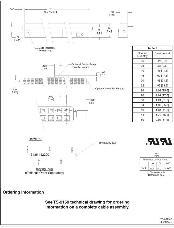
2 mm x 2 mm for 1 mm Pitch Cable, Cable Assembly Connector
